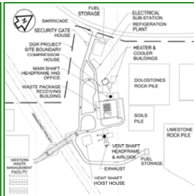
Figure 12-2 – Surface Layout (Operations Phase)
