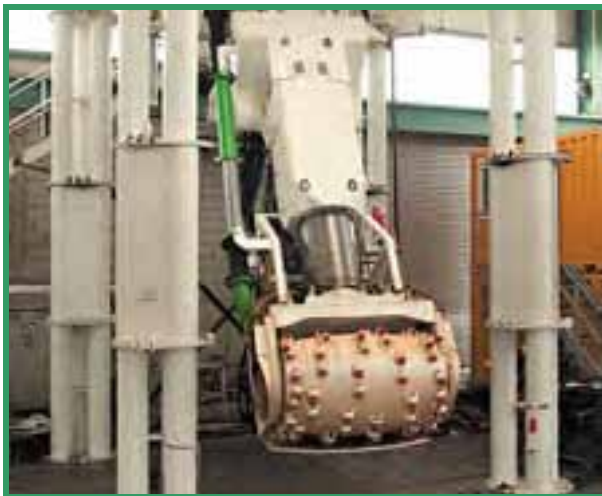
Figure 6-6 – Example of Vertical Shaft Sinking Machines (Herrenknecht, 2007)
